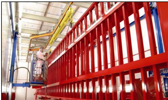
Production line spraybooth at Fruehauf
